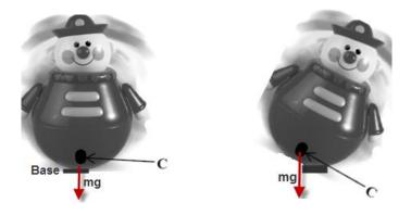
Note that the weight of an object always acts through the centre of gravity (indicated by C in both diagrams).
