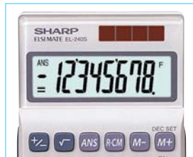
Liquid crystal display in a pocket calculator Reproduced with kind permission of Sharp Consumer Electronics.
