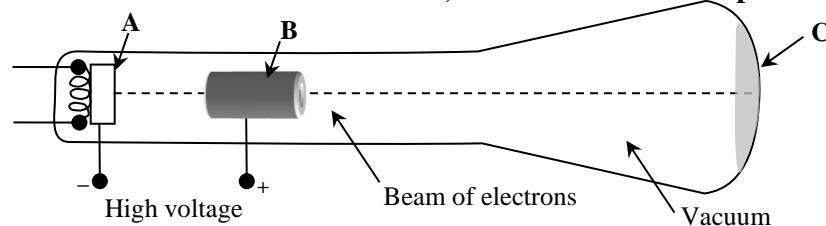
The diagram shows a simple cathode ray tube, which produces a beam of electrons by thermionic emission.
