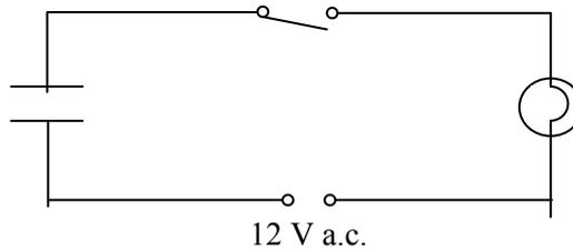
**The diagram above shows a circuit with a bulb, switch, capacitor and a 12 V a.c. power supply.**
