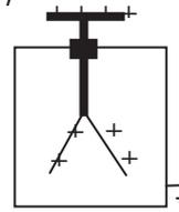
**The diagram shows a positively-charged electroscopes.**
