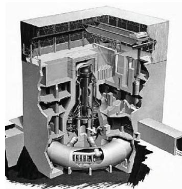
The Fukushima nuclear reactor continued to generate heat even after the chain reaction was stopped because of the radioactive decay of the isotopes created during nuclear fission. This decay cannot be stopped and the resulting heat must be removed by circulating cooling water through the reactor core.
