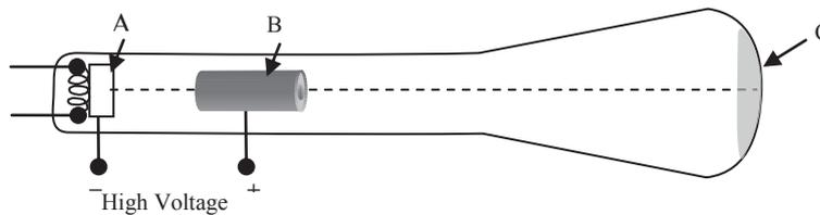
**The diagram shows a simple cathode ray tube.**
