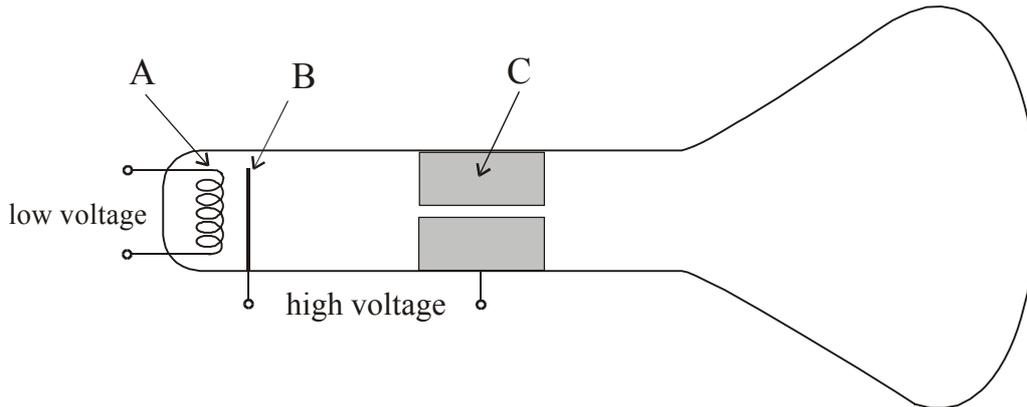
A = (heating) filament/coil, B = cathode, C = anode      **6 + 2 × 3**
